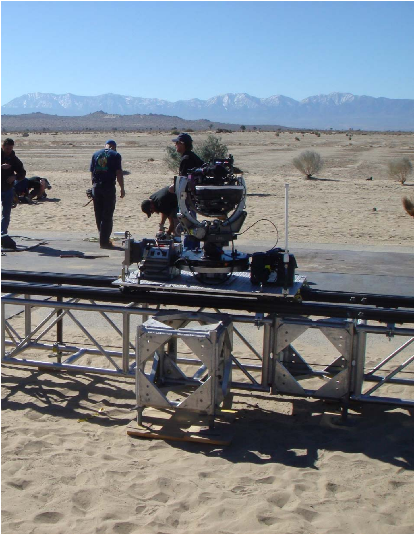
Fastrack clamped to the chords of 20.5" truss.
