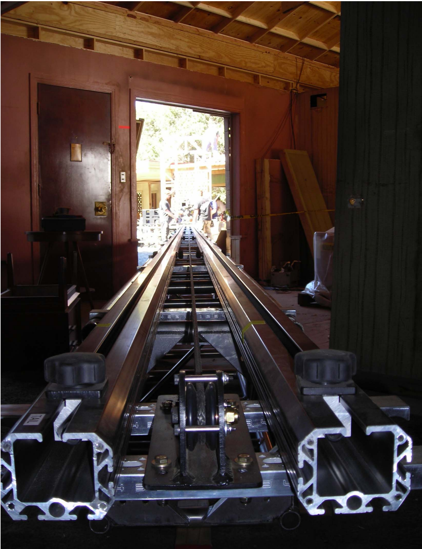
End view of Fastrack grappled to 20.5" truss.
